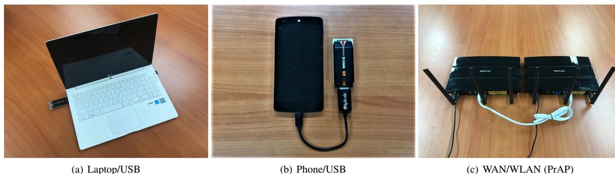
Figure 2. Three ways ways of setting up a rogue AP (rAP), using a universal serial bus (USB)-based wireless interface (along with the built-in wireless interface) as in (a) with a laptop and (b) with a phone, and using a physical layer connector of two routers (PrAP) as in (c).
