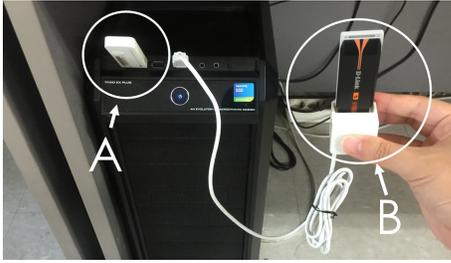
Figure 10. Hardware setting of the desktop PrAP-Hunter. A is a wireless interface that is connected to the target AP and generates traffic, and B is the wireless interface that sends interference signals through 2.4GHz channels.
